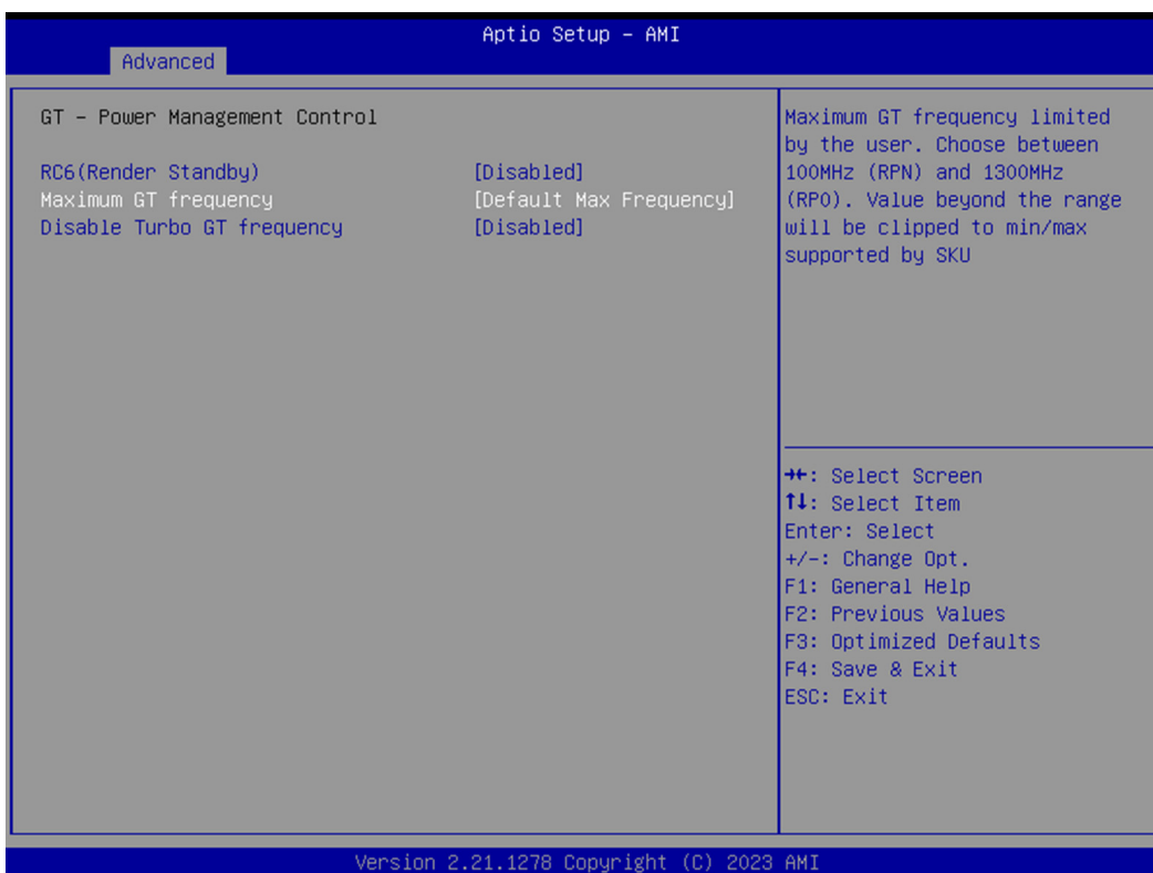
Figure 4.9 GT – Power Management Control
