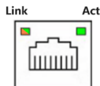
Figure 3.2 RJ45 LAN Connector Layout
