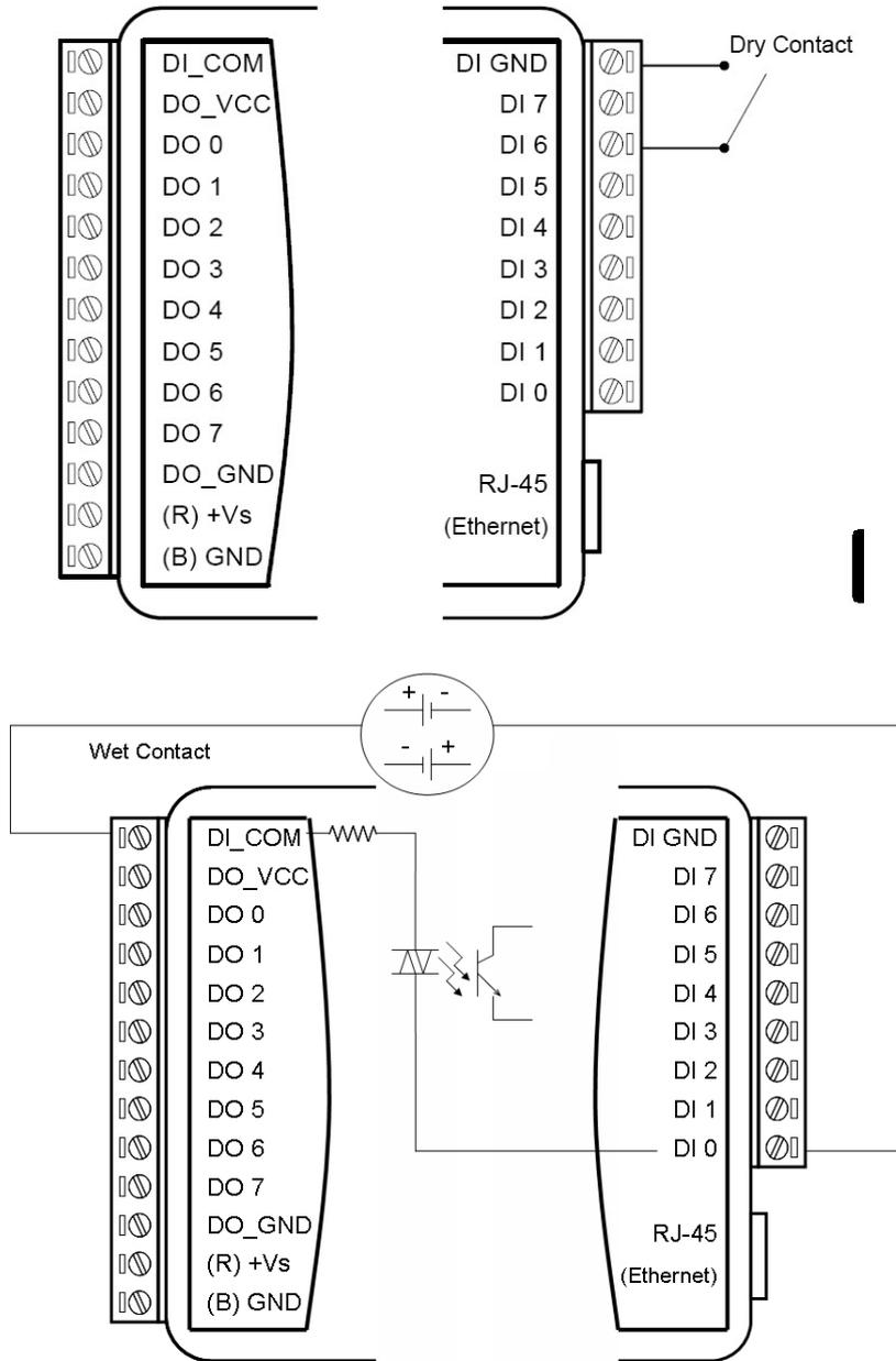
**Figure 5.7 ADAM-6052 Digital Input Wiring**
