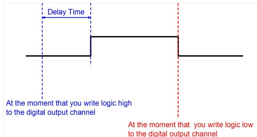
**Figure 6.13 Graph Explaining Low to High Delay Output Mode**
