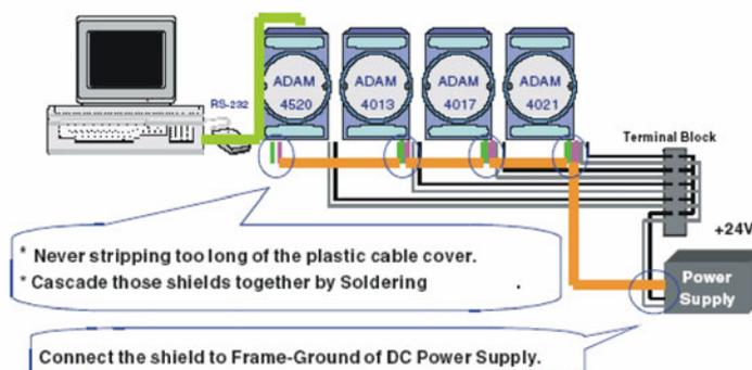
**Figure C.11 System Shielding**
