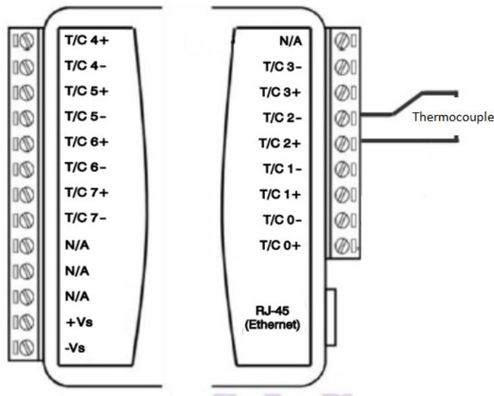
Figure 4.9 ADAM-6018+ thermocouple wiring
