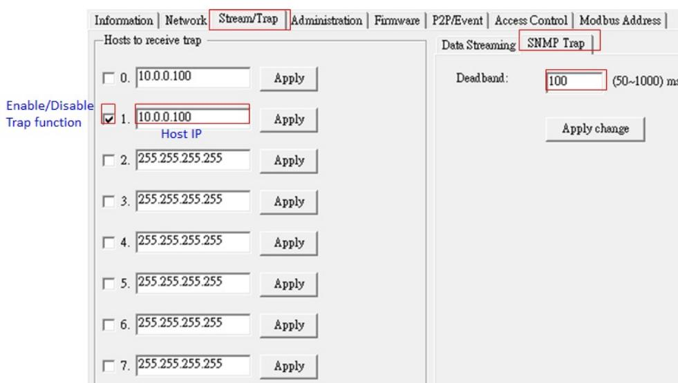
Figure 7.3 Trap Configuration Using Adam/Apax .NET Utility
