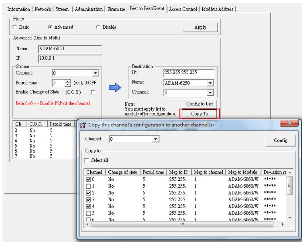
**Figure 6.20 Copy One Setting to Other Channels**
