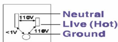
**Normal Mode:** refers to defects occurring between the live and neutral conductors. Normal mode is sometimes abbreviated as NM, or L-N for live - to - neutral.
