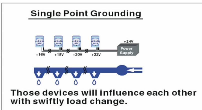
Figure C.7 Single-Point Grounding
