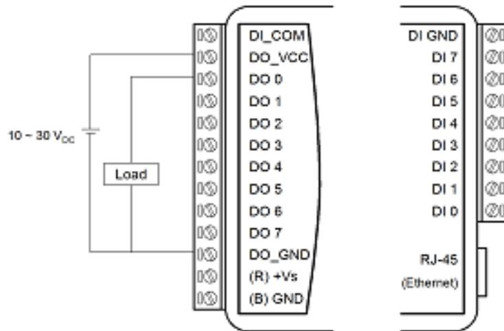
Figure 5.8 ADAM-6052 Digital Output Wiring
