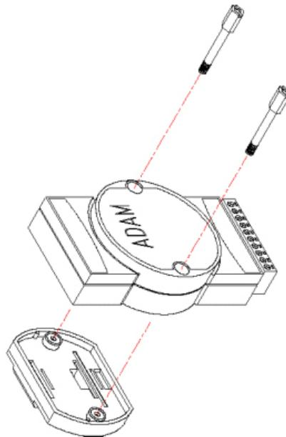
**Figure 3.3 How to Fix a Module on the DIN Rail Adapter**
