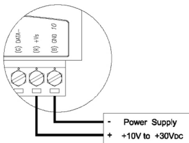
Figure 3.5 How to Connect the Module Power Wires
