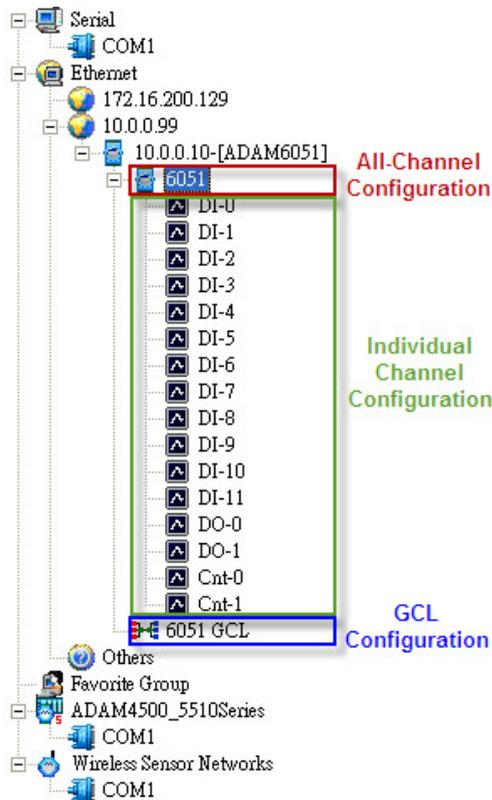
**Figure 6.5 All-Channel, Individual Channel, and GCL Configuration Controls**
