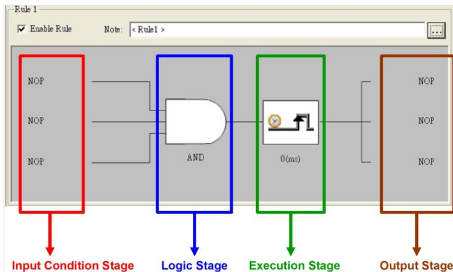
Figure 8.2 Four Stages for One Logic Rule
