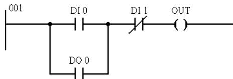
**Figure 8.23 Ladder Diagram for On/Off Control**
