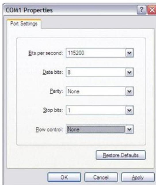
Figure 9 Hyper Terminal Settings for Terminal Setup
