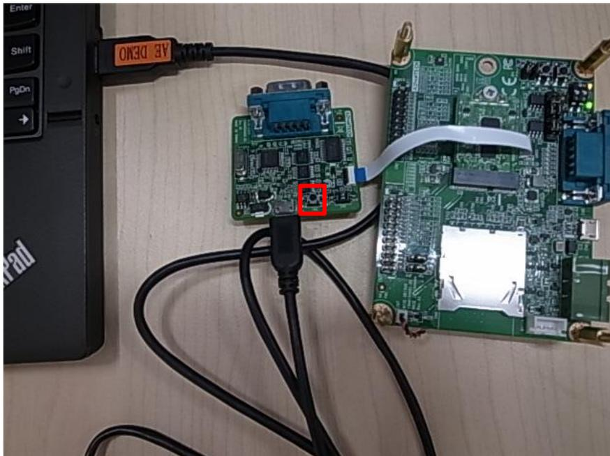
Open the corresponding COM port in serial program, ex: Tera Term. Set baud rate to 115200.
