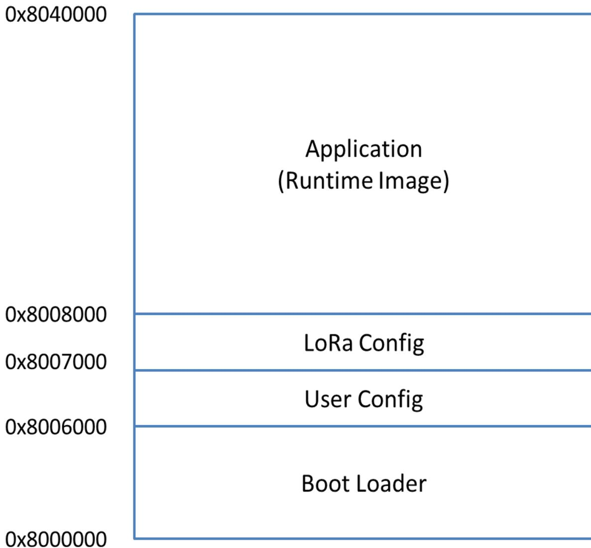
Boot Loader occupies the first 16 kilo-bytes starting at 0x8000000. LoRa Config partition is used to store LoRa parameters, which occupies no more than 4 kilo-bytes. All user own parameters should be written into User Config partition, for which another 4 kilo-bytes are reserved. Application (Runtime image) partition is where users' application is stored, up to 224 kilo-bytes can be used.
