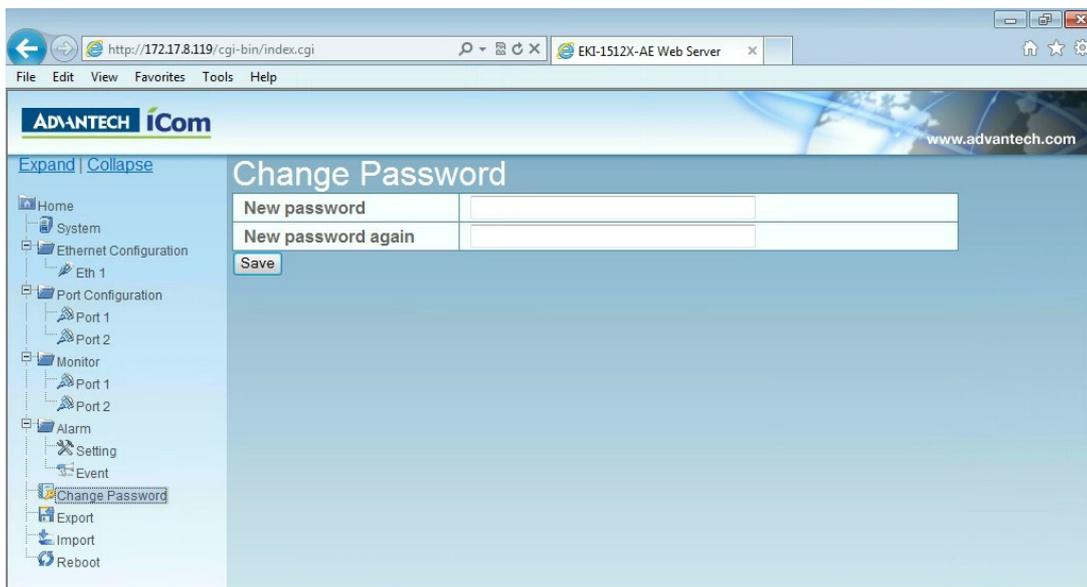
If you want to disable the password protection, just change the password to the default “None” (leave the new password column blank), Be sure to press the “Save” button and reboot the serial device server to make the change effective.
