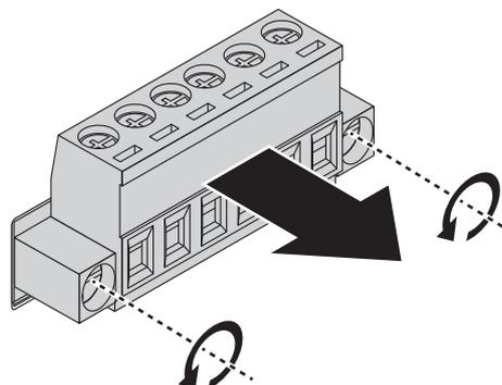
**Figure 2.20 Removing a Terminal Block**
