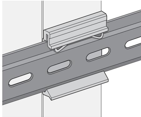
**Figure 2.2 Correctly Installed DIN Rail Kit**
