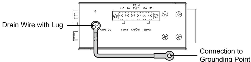
**Figure 2.15 Grounding Connection**
