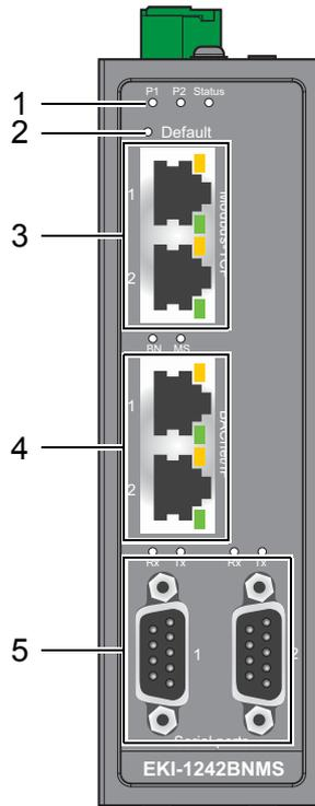
Figure 1.1 Front View (EKI-1242BNMS/EKI-1242IBNMS)
