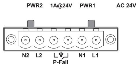
**Figure 2.19 Terminal Receptor: Relay Contact (EKI-1242BNMS/EKI-1242IBNMS)**
