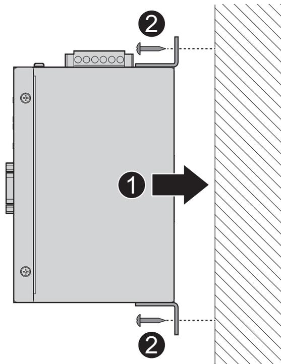
**Figure 2.6 Wall Mount Installation**
