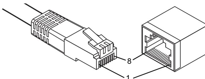
**Figure 2.7 Ethernet Plug & Connector Pin Position**
