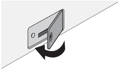
**Figure 2.12 Closing the Component Cover**
