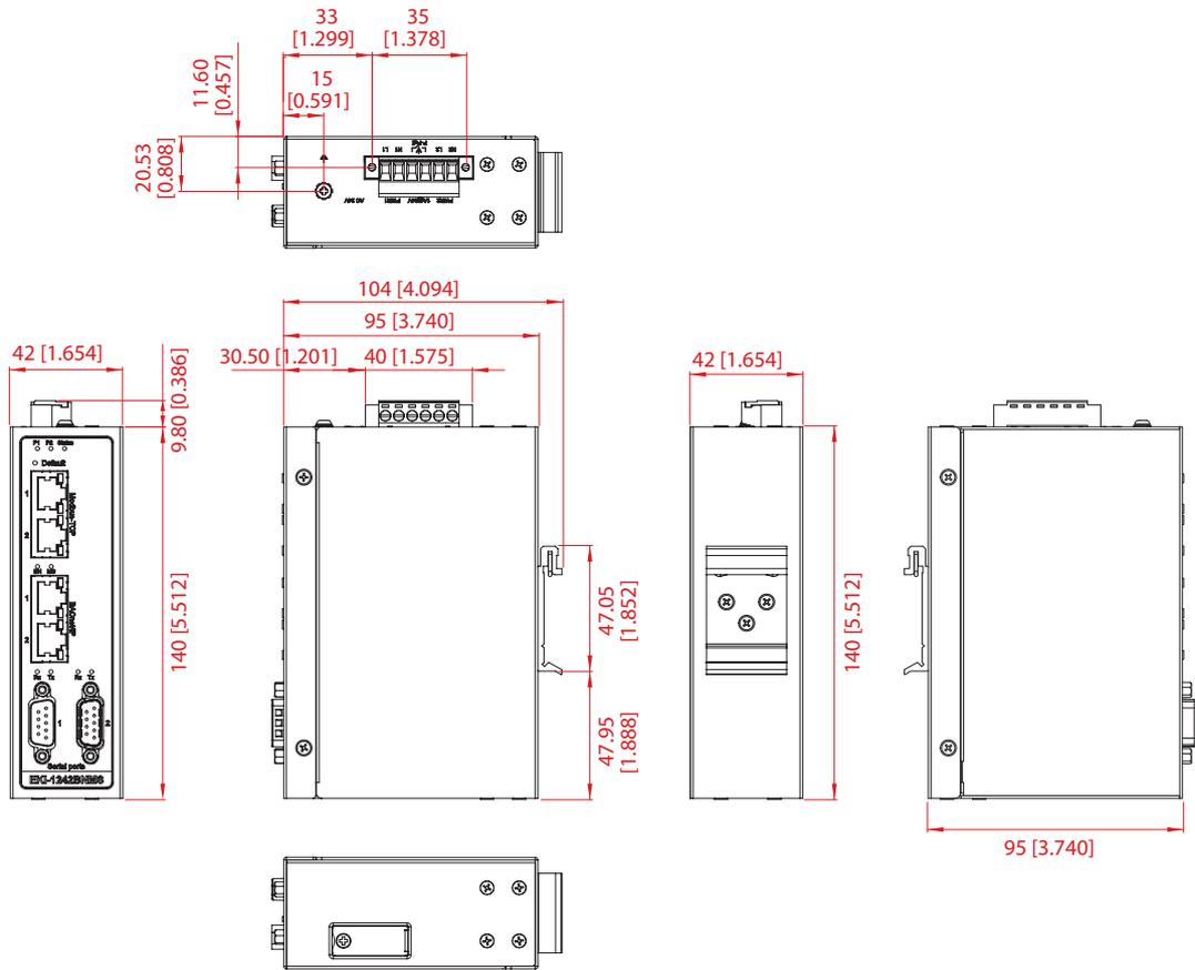
**Figure 1.9 Dimensions (EKI-1242BNMS/EKI-1242IBNMS)**
