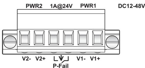
**Figure 2.16 Terminal Receptor: Relay Contact**
