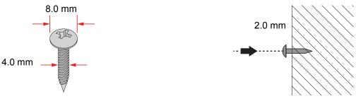
Figure 2.34 Securing Wall Mounting Screws
