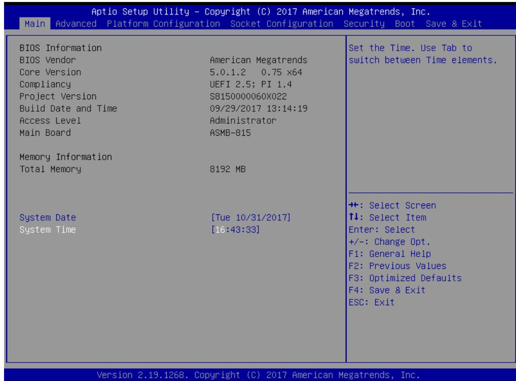
AMI's BIOS ROM has a built-in Setup program that allows users to modify the basic system configuration. This type of information is stored in battery-backed up CMOS so it retains the Setup information when the power is turned off.
