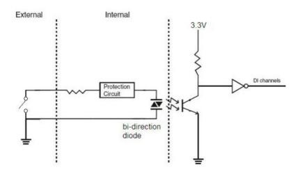
**Figure 2.5 Dry Contact Wiring**
