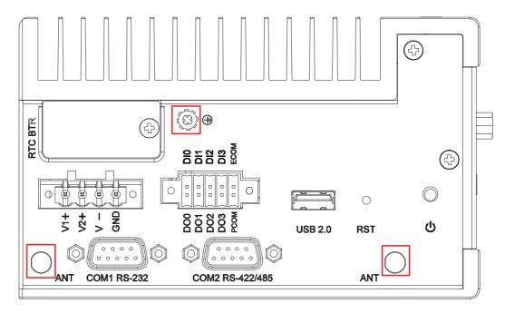
**Figure 3.1 Chassis Grounding Connection**
