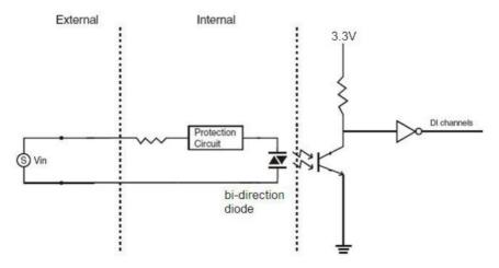
**Figure 2.4 Wet Contact Wiring**
