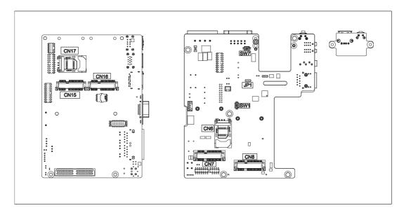
**Figure A.1 Connector & Jumper Locations (front)**
