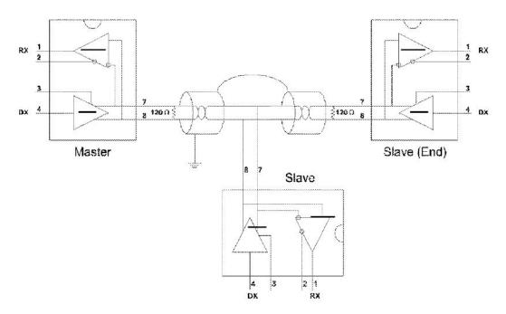
Figure E.2 Termination Resistor Locations
