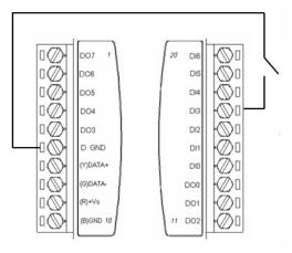
Figure 3.14 ADAM-4150 Digital Input Dry Contact Wiring
