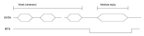
Figure E.3 RS-485 Data Flow Control with RTS
