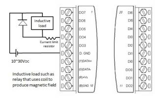
Figure 3.16 ADAM-4150 Digital Output with Inductive Load Wiring
