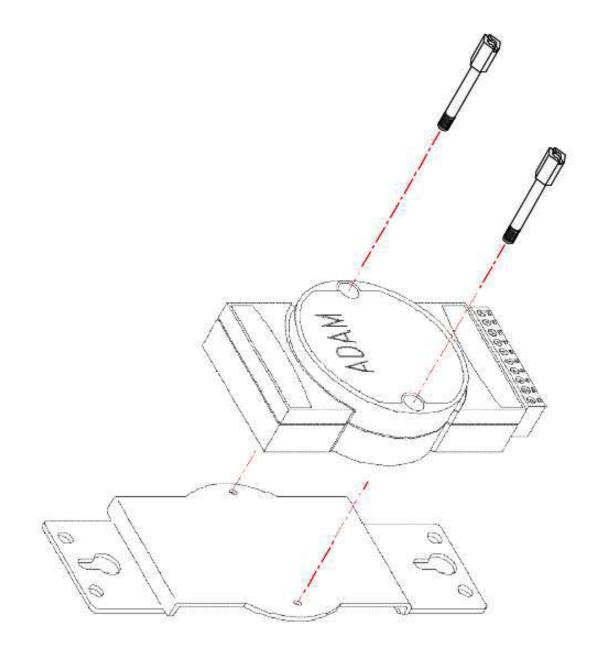
Figure C.4 Installation onto the Panel Mount
