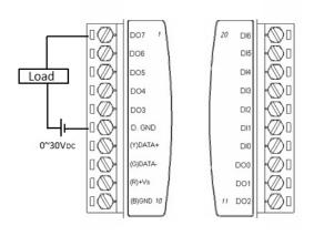
Figure 3.15 ADAM-4150 Digital Output Wiring
