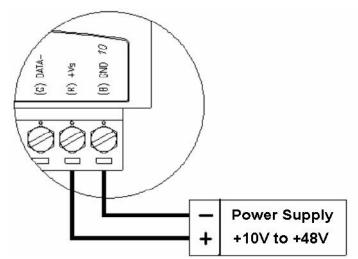
**Figure 2.1 Power Supply Connections**
