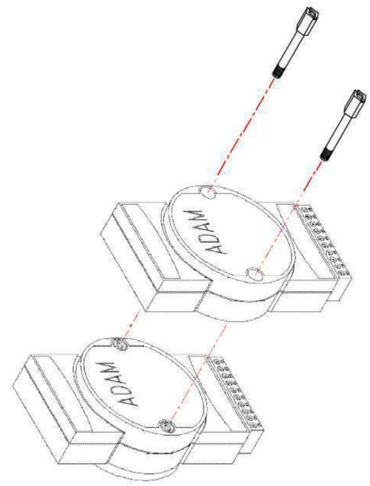
Figure C.5 Piggyback Stack Configuration
