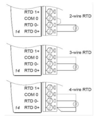
Figure 3.22 ADAM-4115 RTD Input Wiring
