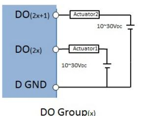
Figure 3.25 Process to Trigger Two Actuators at the Same Time
