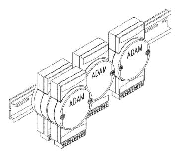
ADAM modules may be mounted on any panel, the provided brackets, DIN rails, or they may be piggybacked on top of each other. The RS-485 network, together with screw-terminal plug connectors, allows for system expansion, reconfiguration, and repair without disturbing the wiring.
