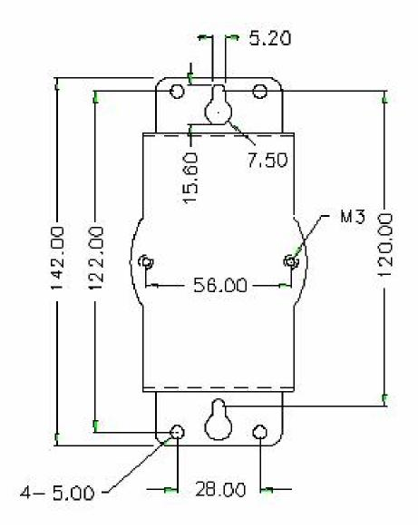
Figure C.3 Panel Mounting Bracket Dimensions
