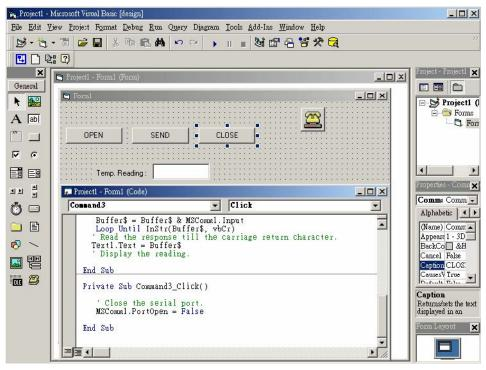
10. Run the project, click **OPEN** to open COM1, then click **SEND** to send the get temperature reading command. Now, you will find the reading the same as the displayed format shown in the following image:
