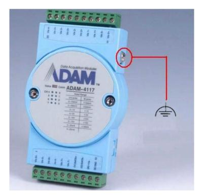
Figure 2.3 Ground Connector on an ADAM-4117
