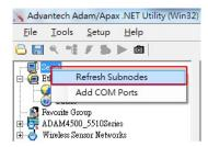
3. The COM port for the module will be shown in the utility; select it and change the baud rate to 9600 and click Apply
